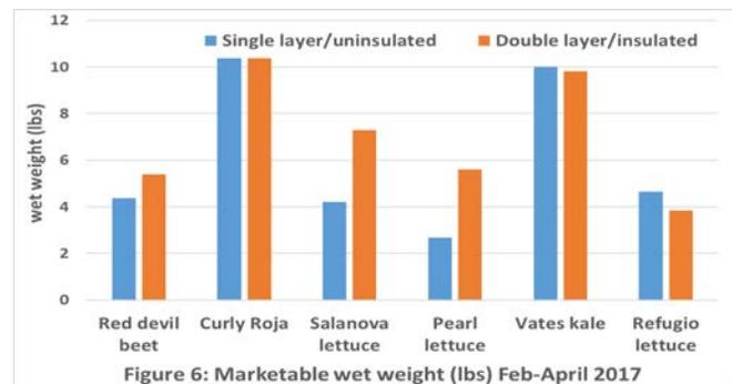
Figures 1-6: Comparison of plant growth between single layered uninsulated and double layered insulated high-tunnel greenhouse structures.
